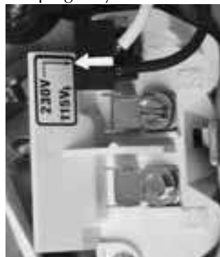
Figure 4A - Voltage Change Plug Set for 230 Volts
