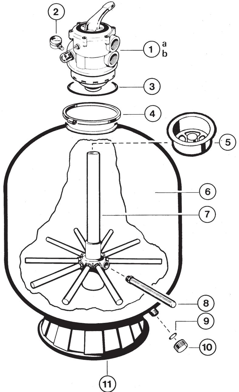
3. Loading sand media. Filter sand media is loaded through the top opening of the filter.
