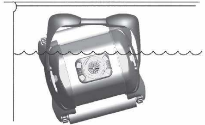
Incorrect waterline height
