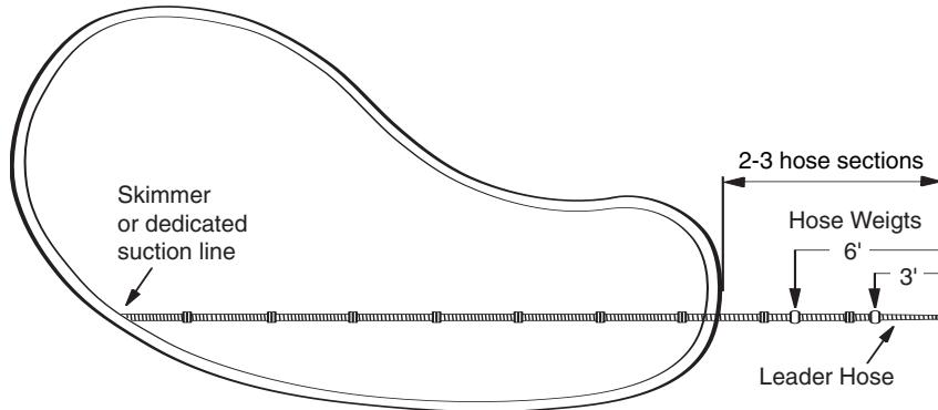
**Note:** For pools less than 5 feet deep, remove weight from leader hose and position weight on standard hose four feet from Polaris.
