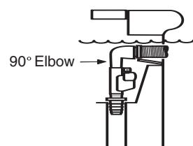
On some skimmers it may be necessary to install an elbow connector to keep the hose from kinking. For deep skimmers, install the 45-degree elbow between the flow regulator and the hose. For shallow skimmers, use the 90-degree elbow.
