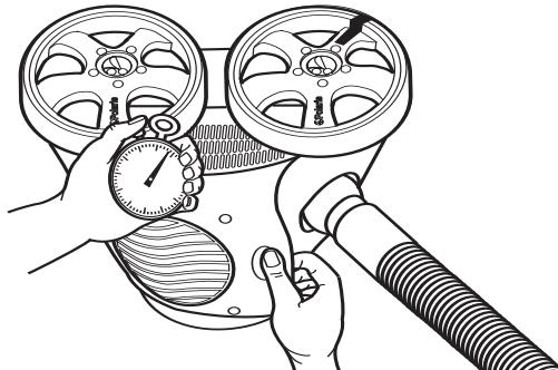
**If count is less than 30 RPM:**
