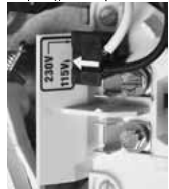
Figure 4B - Voltage Change Plug Set for 115 Volts
